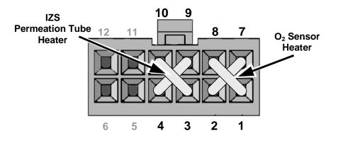
Figure 2-5: Typical Set Up of AC Heater Jumper Set (JP2)
